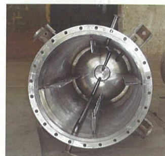
种子罐夹套内部结构图 inner structure illustration of seed Tank Jacket
